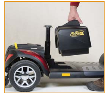
Step 2: Pull out the battery pack!
