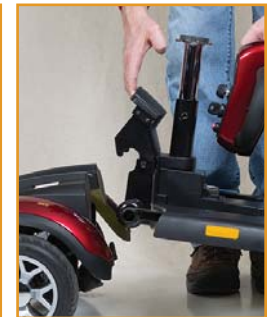
Step 4: Pull forward on the drivetrain release lever to separate the front and rear frame sections!
