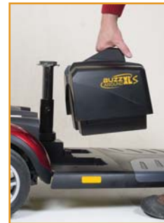
Step 2: Pull out the battery pack!
