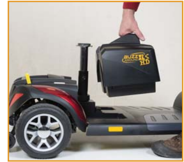
Step 2: Pull out the battery pack!
